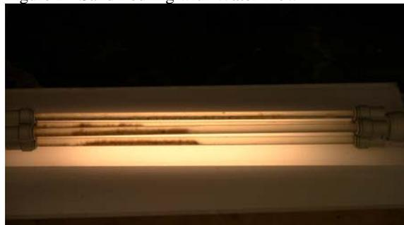
Figure 3 - Sand Fouling as Ice Pig Enters
