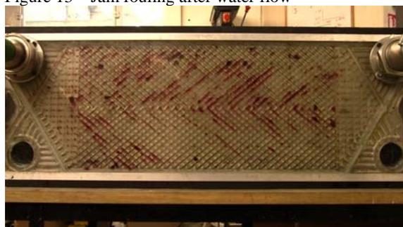
Figure 14 – Jam fouling shortly after ice pig entry
