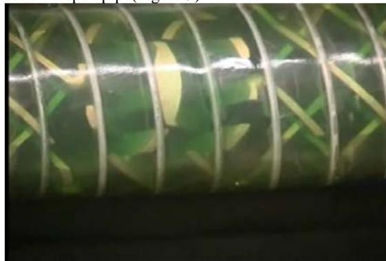
Figure 6 - Sulzer Static Mixer with Detergent
