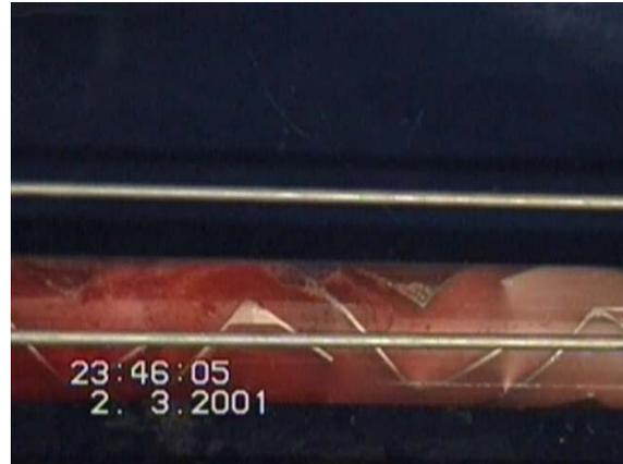
Figure 10 – Kennix mixer during pig insertion
