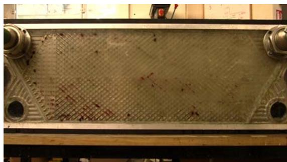
Figure 15 – Jam fouling at the end of the ice pig
