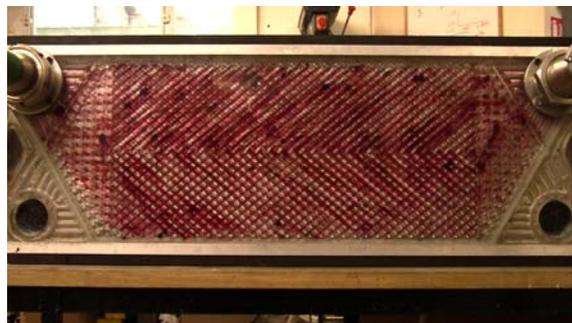
Figure 12- Jam fouling before water flow
