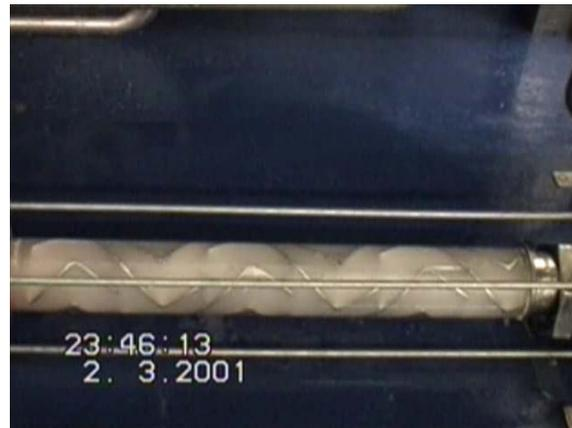
Figure 11 - Kennix Mixer with ice pig
