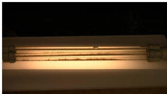
Figure 2 - Sand Fouling with Water Flow
