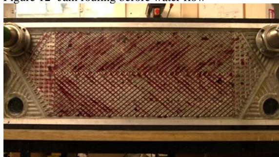
Figure 13 – Jam fouling after water flow
