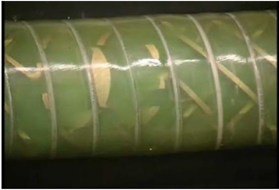
Figure 7 - Sulzer Static Mixer as Pig Enters
