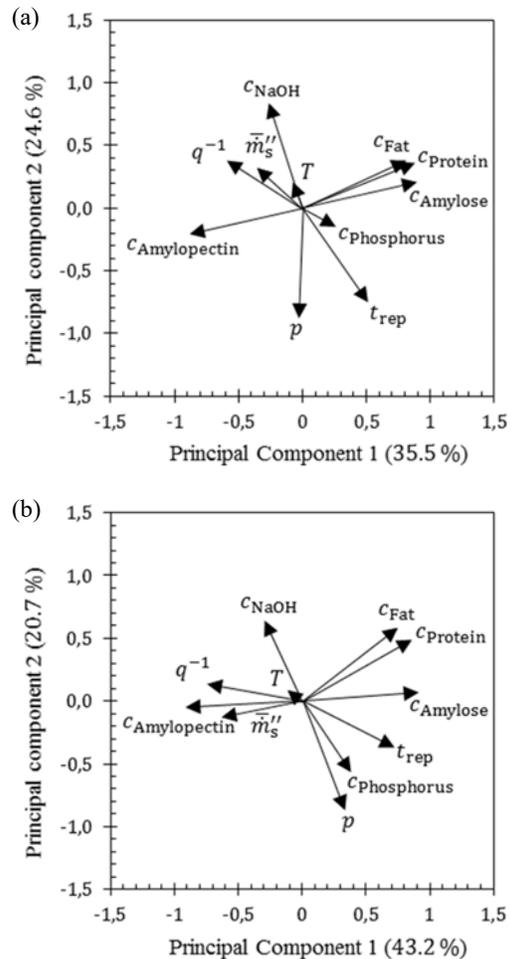
Fig. 6. Principal component plot of plane channel experiments (a) and falling film experiments (b);  $t_{\text{rep}}$  was set to 1800 s, when no cleaning occurred
