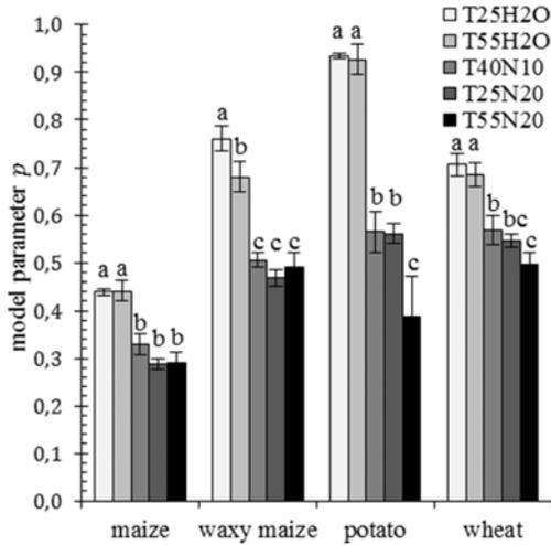
Fig. 2. Maximum intensity capacity  $p$  in plane channel flow; Mean  $\pm$  SD values ( $n = 3$ ); values with different letters within a starch differ significantly at  $P < 0.05$
