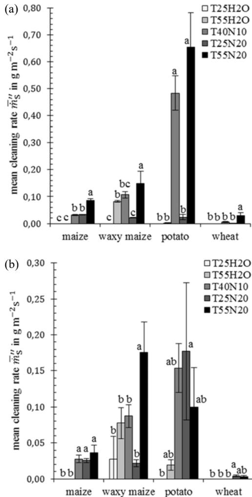
Fig. 5. Mean cleaning rate  $\bar{m}_s''$  in plane channel flow (a) and falling film setup (b); Mean  $\pm$  SD values ( $n = 3$ ); values with different letters within a starch differ significantly at  $P < 0.05$ ;  $\bar{m}_s'' = 0$ , when no cleaning occurred
