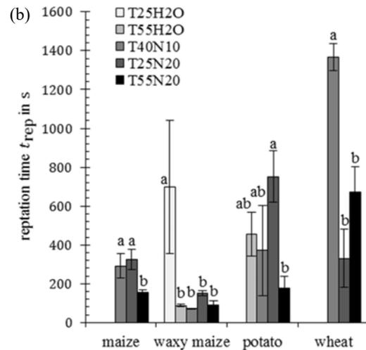
Fig. 4. Reptation time  $t_{rep}$  in plane channel flow (a) and falling film setup (b); Mean  $\pm$  SD values ( $n = 3$ ); values with different letters within a starch differ significantly at  $P < 0.05$ ;  $t_{rep}$  is not shown, when no cleaning occurred for 1800 s
